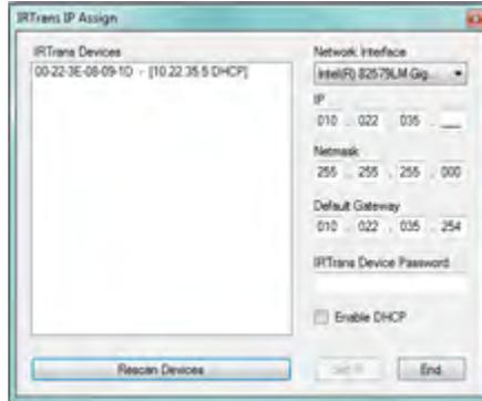
IPAssign searches the network for IRTrans devices and sorts them according to MAC addresses. An entry marked with „DHCP“ means that this device obtained its settings from a DHCP server. After selecting an IRTrans device its settings can be changed. Writing the settings to the device („Set IP“) requires the correct device password to be entered.
