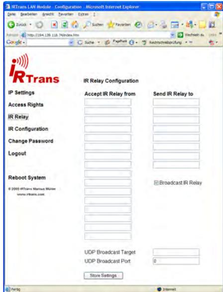
The UDP Broadcast fields are only used for modules with integrated IR Database. They define to which address and port formatted IR receive data has to be sent. The precise format of these telegrams is configured via the IR database.
